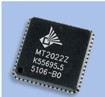
MT2022 Single-Chip Broadband Tuner
